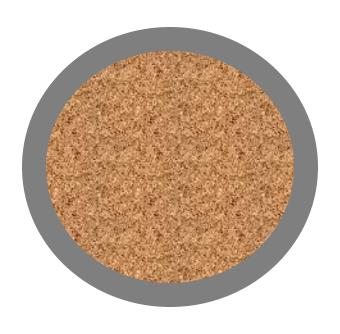
RAP aggregate with oxidized binder film
